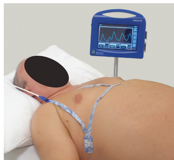
Figure 1 A non-invasive respiratory volume monitor (ExSpirom; Respiratory Motion, Inc.) that provides continuous, real-time, non-invasive measurements of minute ventilation, tidal volume and respiratory rate. This photograph shows standard electrode placement on an obese patient (not the patient reported here; body mass index, 36.7kg/m 2 ). One electrode is placed at the sternal notch, another on the xiphoid and the third in the right mid-axillary line at the level of the xiphoid.
