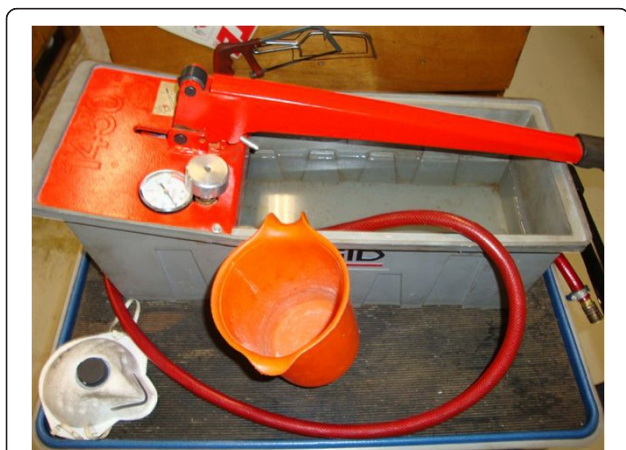
Figure 1 Pressure test pump.
