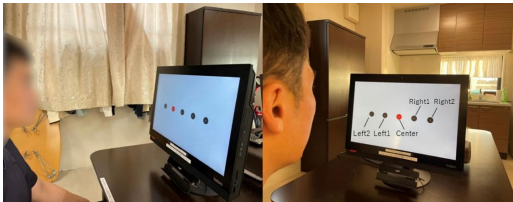
Fig. 2 Scenario for the evaluation of eye movements. Eye movements require observation of five objects on the PC display that were detected using the eye tracker
